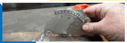
Visual testing should be conducted in accordance with VT standards or procedures by a qualified visual inspector. ISO 17637 is an International Standard that delineates the visual testing procedures for fusion welds in metallic materials.
