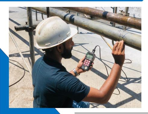
Ultrasonic Thickness Gauges are precise tools that measure material thickness, especially metals, using sound waves without causing damage. They work by sending high-frequency waves through a material and measuring the time for them to return, calculating thickness based on sound speed.
