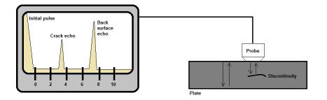
Ultrasonic testing (UT) employs highfrequency sound waves to assess materials, detect flaws, and characterize their properties. Using short pulse waves typically between 0.1-15 MHz (up to 50 MHz in some cases), UT is a versatile nondestructive testing method widely utilized across various industries.
