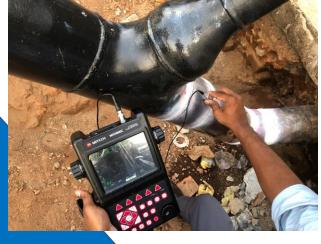
Ultrasonic testing offers numerous advantages, including deep flaw detection, high sensitivity, accessibility from one side, accurate flaw characterization, non-hazardous operation, and quick results. However, it requires skilled technicians, may yield false positives, and faces challenges with rough or irregular objects, requiring couplants for conventional tests and potentially reduced sensitivity for certain flaws.
